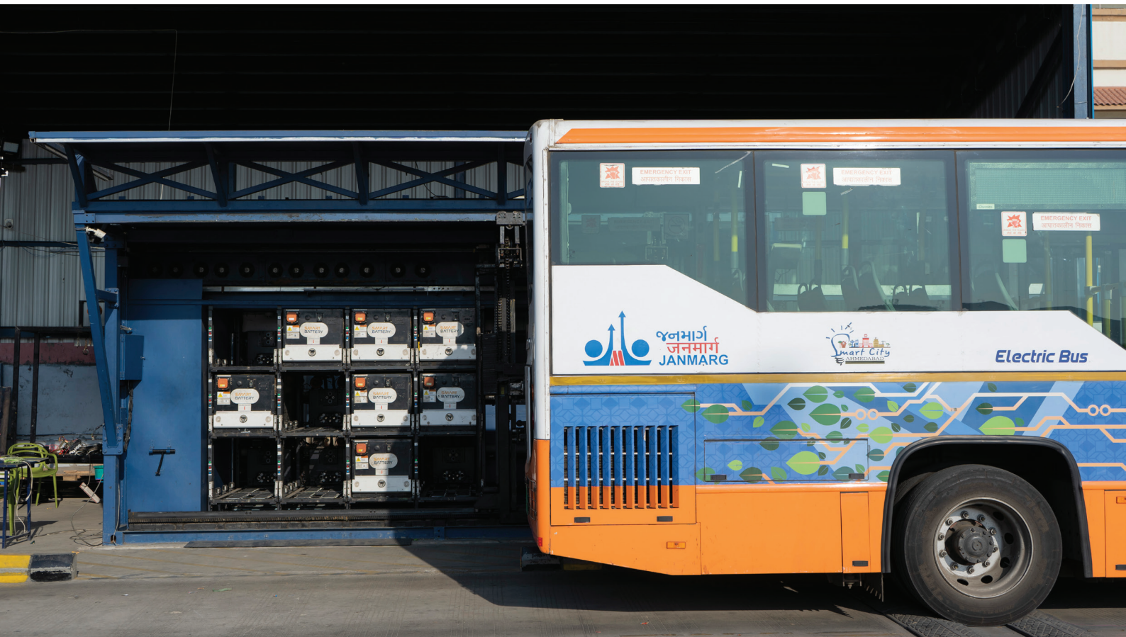
Electric bus with ‘battery swap’ technology developed by SUN Mobility
