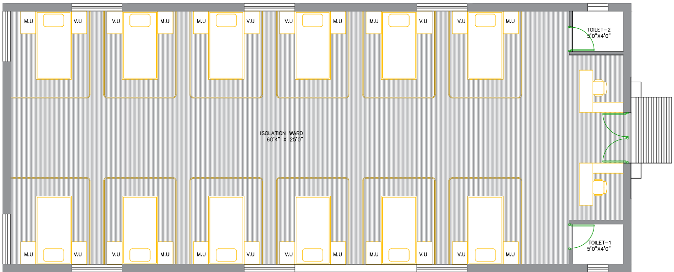
Figure 9 : ICU layout for patients with severe symptoms of COVID-19 in community halls and marriage halls
