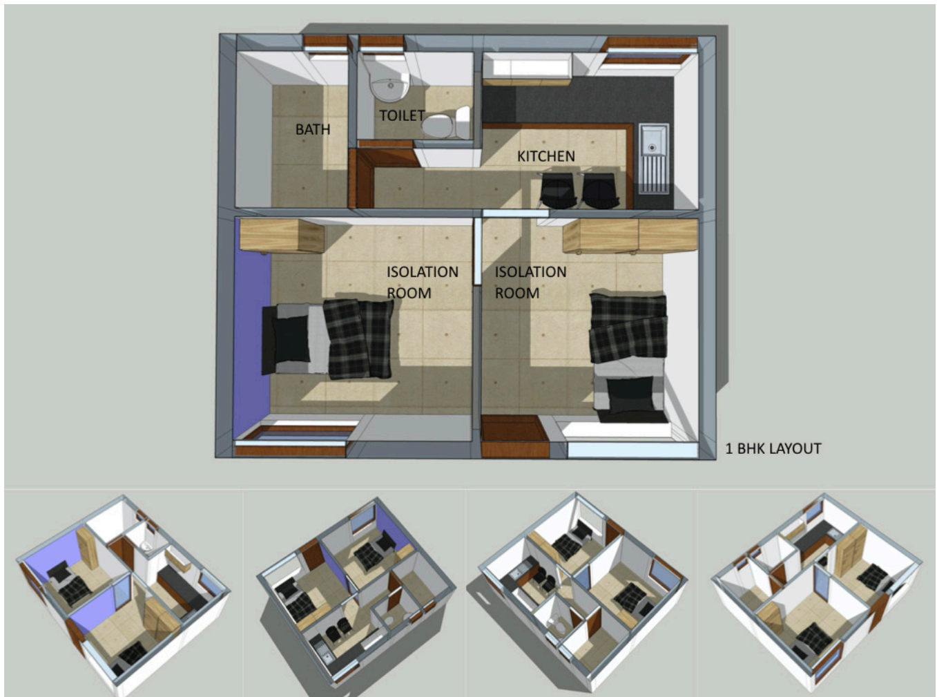
Figure 12: 3D rendering of a general ward layout for patients with asymptomatic, mild, or moderate COVID-19 symptoms in a 1 BHK vacant home
